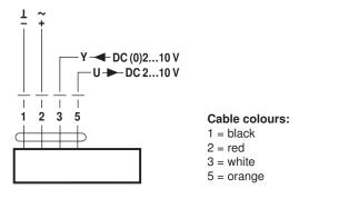
Override control (frost protection circuit)
