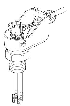
**How to specify** Conductivity probe with austenitic stainless steel body and probe tips, PFA tip insulation, suitable for steam boiler operation up to 32 bar g @ 239°C.
