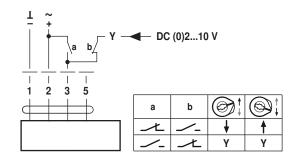
Override control (frost protection circuit)
