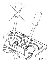
**Note:** Do not drill into the base as this creates metal shavings which can create electrical hazards and damage the device. Drilling voids the warranty.
