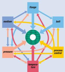
Maximum temperature and pressure values alone can not define a material's suitability for an application. These limits are dependent upon a multiplicity of factors as shown in the diagram opposite. It is always advisable to consider these factors when selecting a material for a given application.
