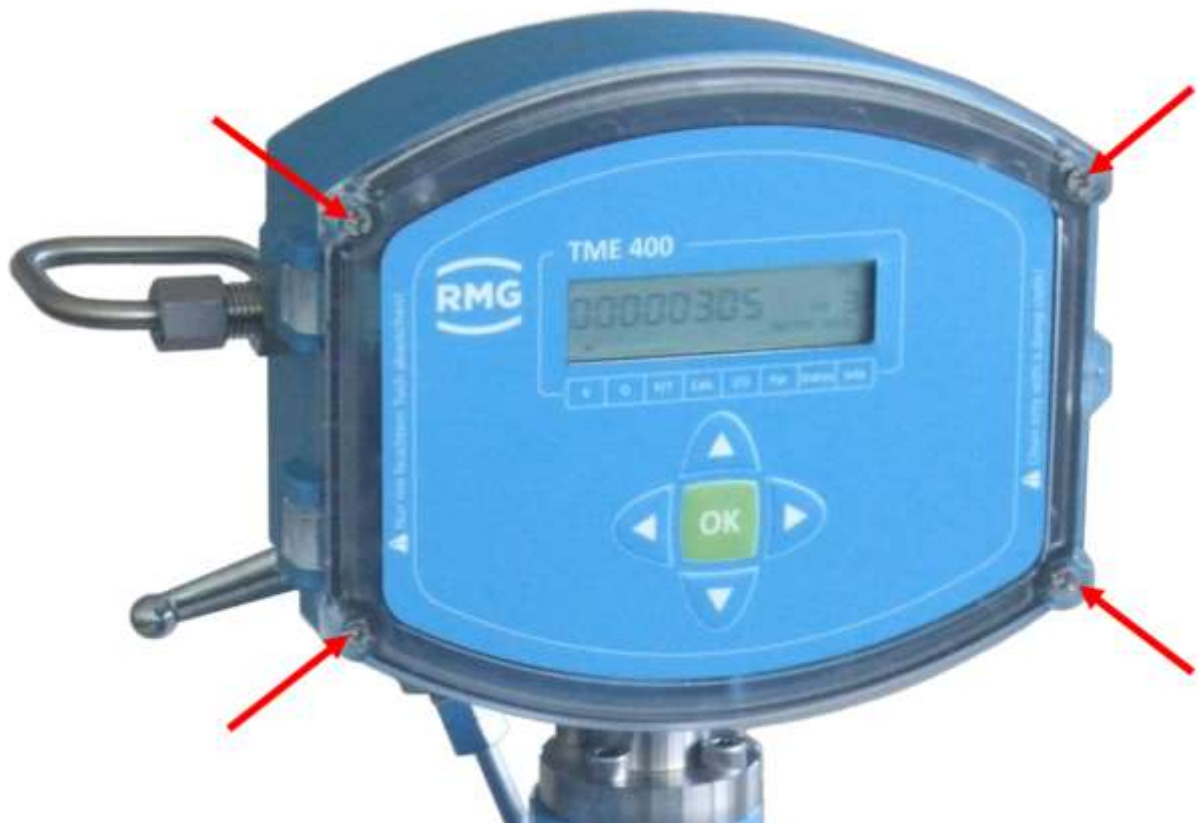
Figure 3: Unscrewing the screws to open the cover
