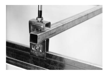
7. Slide A centre bracket onto the square bar, mount the outlet reducer through the A centre bracket and lightly tighten the nut. Adjust location of the centre bracket and the side B brackets until desired location of the outlet reducer is achieved. Firmly secure the side B brackets by tightening the screws to a torque of 5 Nm/4 ft-lbs.
