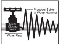
Water hammer is usually recognized by a banging or thumping in water lines when valves are shut off. Although this is an easy way to recognize the problem, water hammer doesn't always make these telltale noises.
