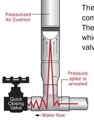
The most effective means of controlling water hammer is a measured, compressible cushion of air which is permanently separated from the water system. The Hydra-Rester® employs a pressurized cushion of air and a two o-ring piston, which permanently separates this air cushion from the water system. When the valve closes and the water flow is suddenly stopped, the pressure spike pushes
